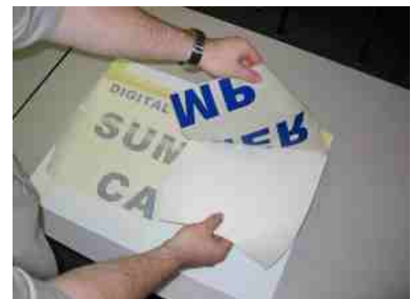
Removing Liner Using Scissors Method
